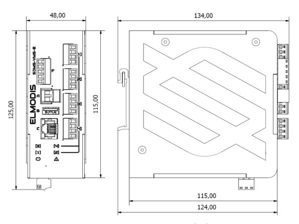
Fig 6. SDMS-VMS-E module dimensions [mm]
