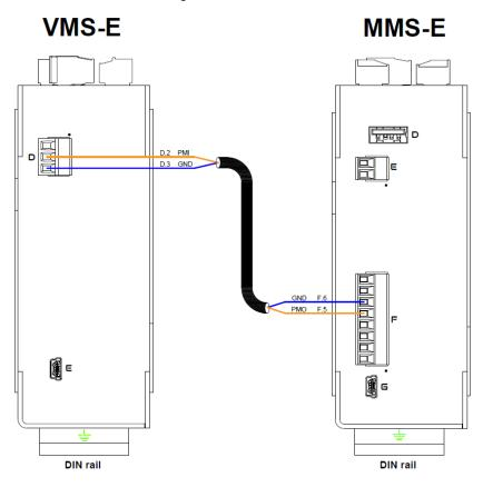
Fig 22. SDMS-MMS-E connection with SDMS-VMS-E
