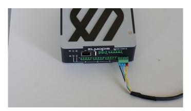
Fig 13. Example connection of sensor directly to the module
