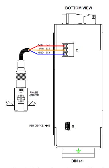
Fig 17. Connecting the phase marker to the D connector of the module
