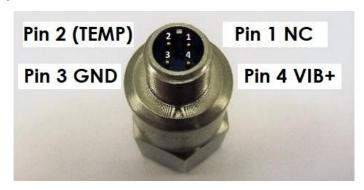
Fig 15. Pin layout on M12 IEC60947-5-2 type connector in the sensor
