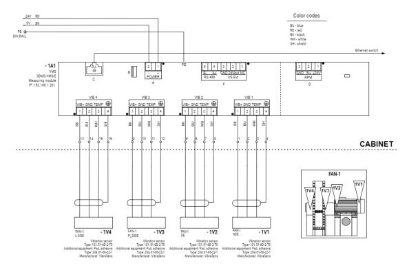
Fig 5. CAD drawing example of connections to the module connectors, including marking standards
