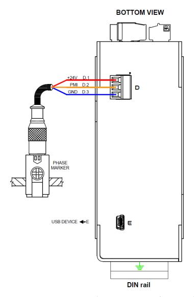
Fig 4. Basic measurement scheme of SDMS-VMS-E module (bottom view)
