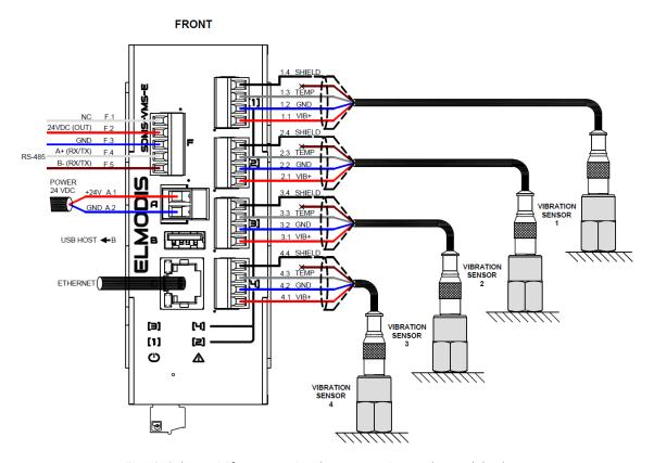
Fig 10. Schematic for connecting the sensor wires to the module plugs.
