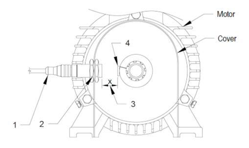
Fig 20. Mounting the inductive sensor
