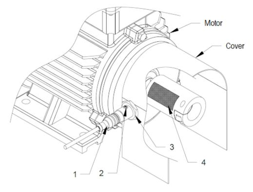
Fig 21. Mounting the optical sensor
