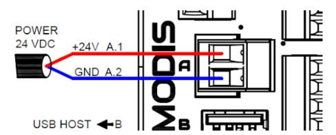
Fig 7. 24 VDC power supply
