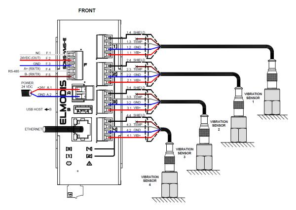
Fig 3. Basic measurement scheme of SDMS-VMS-E module (front view)
